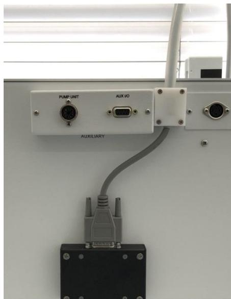
**Fig. 9 and Fig. 10** Mounting the cable guide
